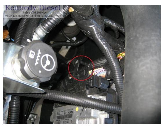
Release the Weatherpack connectors by raising the lever:
