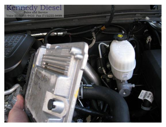
Take the same route back in to place the ECM back in the ECM carrier. Press on the ECM to ensure it fully seats and engages the locking tabs:
