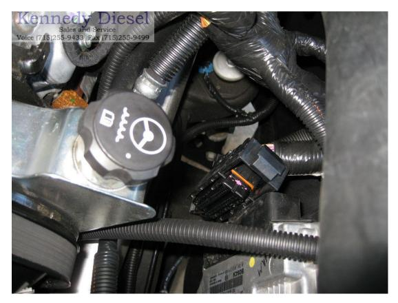
Once the Weatherpack connectors have been disconnected, locate and release the ECM retainer tabs along the top of the ECM carrier. While lifting up on the retaining tabs apply pressure on the ECM by pulling it towards the passenger side of the truck:
