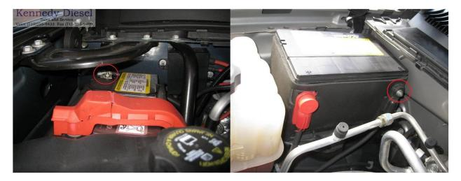
Installers Note - The battery disconnect is standard for any electrical system work and is recommended by GM. It is cheap insurance to protect the system from electrical damage, however in practical experience the ECM swap can be done with the batteries connected with minimal risk. Once the batteries have been disconnected, locate the ECM on the driver's side, near the battery:
