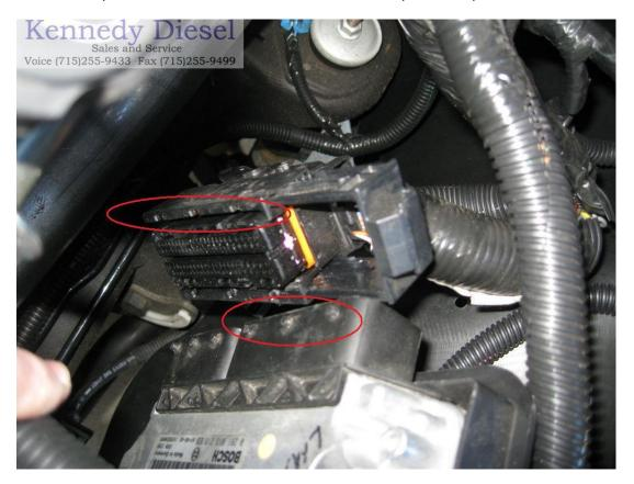
The Weatherpack connectors have slots that must match up with the pins on the ECM connector:
