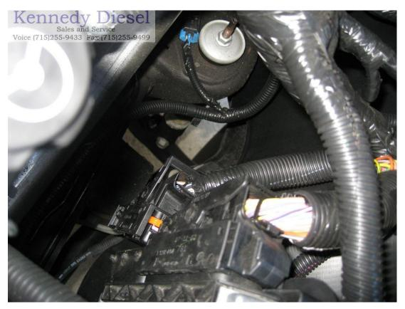
Once the connectors are installed, re-connect the battery ground cables and test starting the truck. There should be no problems starting the engine or check engine lights:
