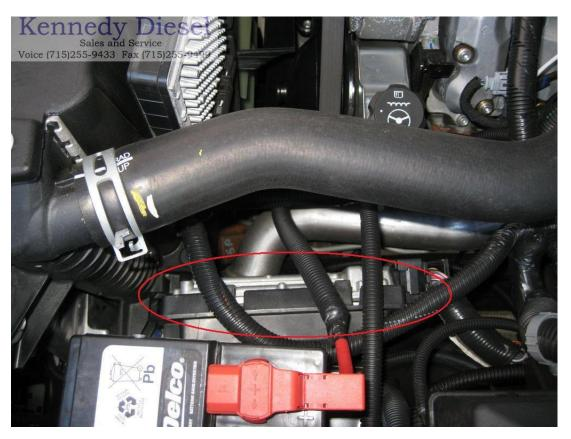
There are two electrical harness bundles using a lever actuated Weatherpack connector that connect the ECM to the main wiring harness:
