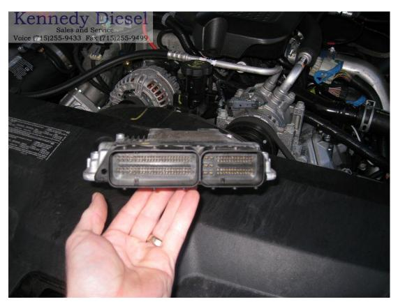
Next install the replacement ECM. The ECM cooling fins should be facing out and the larger ECM connector should be oriented on top upon reinstall:
