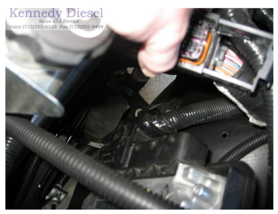
The upper connector is shown above locked in place for reference:
