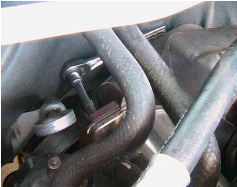
Once the nuts are loose, pry the flange apart. You can use the handle of the ratchet to keep it apart if needed.
