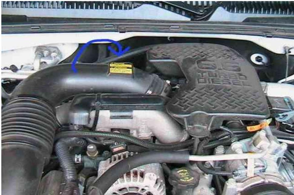
The **third photo** is a more specific location of where the plate is installed. It installs in the flange that connects the exhaust to the EGR (silver horizontal tube). The flange is located near the firewall to the driver's side of the transmission dipstick / beneath the two rubber hoses that come out of the firewall.
