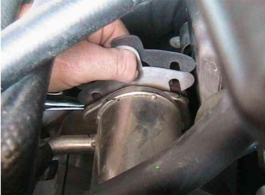
Once the plate is in place, retighten the nuts. Start the engine and feel with your fingers to make sure you don't have an exhaust leak (do this before the engine gets too hot).
