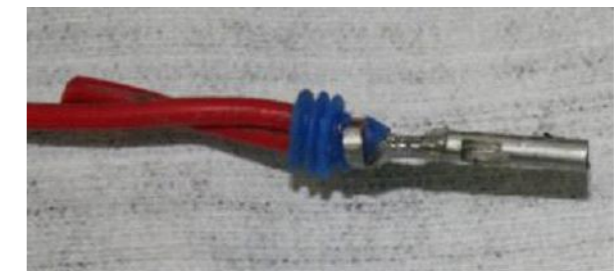
Crimp 2 Wires into each Terminal as shown above
