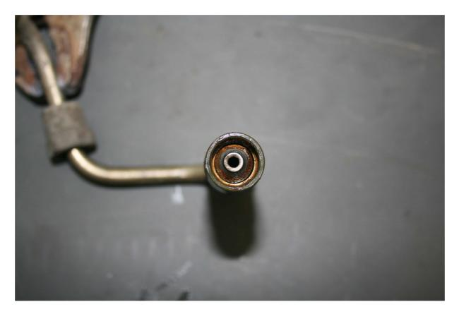
At a glance one would think that a simple cleaning of the tip of the line taper would suffice, but the reality is that this corrosion is on the inside of the line nut in the threads as well as up the shaft of the line around the entire seating ball. The line nut cannot be slid back enough to expose the seating ball so I sectioned one as shown below:
