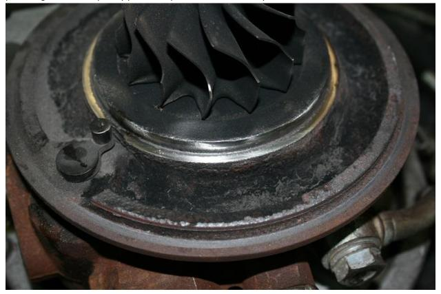
Just for grins I run a flapper wheel on the ID of the unison ring to clean it up a bit but there is typically little to no buildup here.
