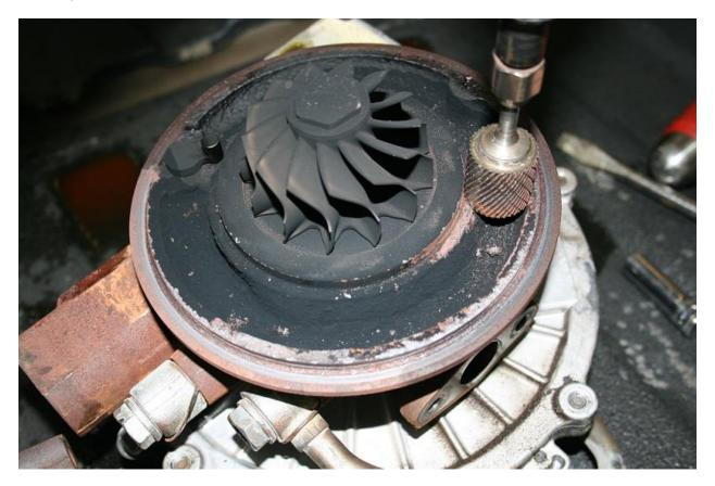
Following the carbide burr I switched to a Roloc type disc. It took a few discs as they wear out quickly.
