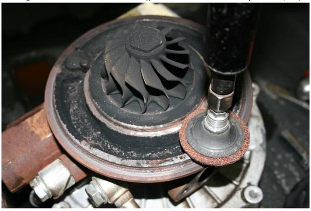
The finished surface has a nice polish to it. I smear this with a liberal coat of dielectric grease to it. The polished finish plus the grease will hopefully prevent repeat corrosion but only time will tell.
